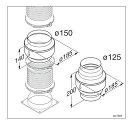
In addition to insulating the exhaust ducting, we recommend that a suitable condensate trap is also installed to collect and evaporate any condensate which may occur. Condensate traps are available for  $\emptyset$  125 mm or  $\emptyset$  150 mm ducting.
